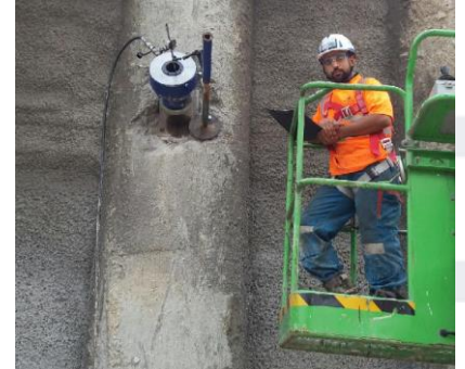
Lift-off test on a threaded block
