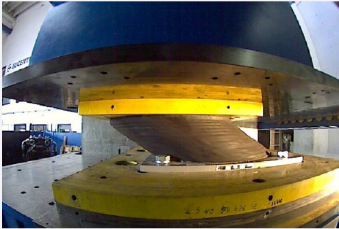
Dynamic and static tests on ISOSISM® HDRB isolators
