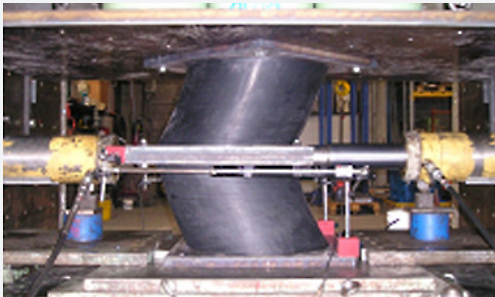
Dynamic and static tests on ISOSISM® HDRB isolators
