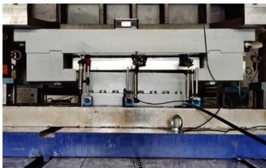
TETRON® DC-SB bearing test for concurrent uplift and rotation at ISOLAB testing facility
